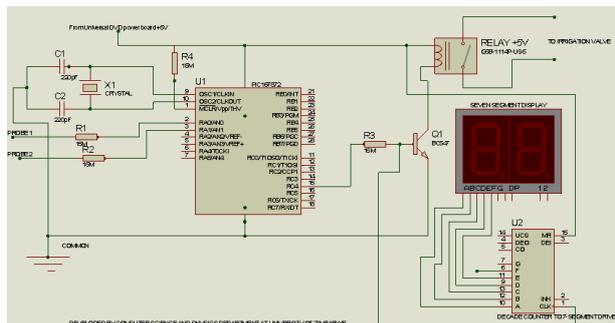
**Figure 1: Soil moisture-based irrigation controller circuit diagram**
