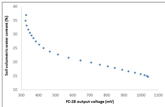
**Figure 3: Relationship between the output voltage and the soil moisture for the FC-28 dielectric soil moisture sensor**
